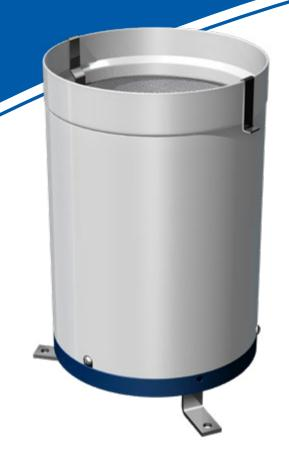
The model **H-3401** is a precision tipping bucket rain gauge used in hydrometeorological applications. Each gauge is calibrated at a rate of 10 mm (4 in) per hour. Maintain accuracy at increased rates of rainfall ranging from 635 mm (0-25 in) per hour. The H-3401 series is available in 0.01 in, 0.1 mm, and 0.2 mm resolution ranges.
